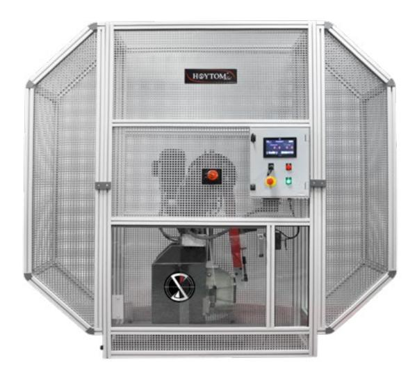
The Hoytom pendulum impact tester has been designed to test metals according to the Charpy or Izod impact testing standards. It is available in capacities from 150 to 750 Joules.
