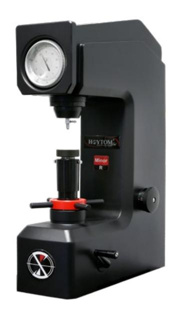
The Minor-R and Minor-S models are quick and simple hardness testers, that enable direct readings to be taken using the Rockwell and Rockwell superficial scales respectively.
