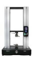
The HM-D model, which is part of the Hoytom LAB series, is made with nominal capacities between 5 and 1000 kN. Its high capacity load cell provides maximum precision across the entire measurement range. It can also be equipped with an extensive range of fixtures, such as tensile grips, T-slotted plates, compression plates, bending fixtures, extensometers, etc.
