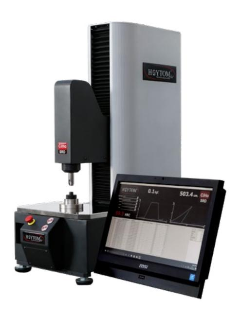
This model has been developed to perform tests using the Rockwell scale (with loads of 60, 100 and 150 kp), and the Rockwell superficial scale (loads of 15, 30 and 45 kp), but can also apply additional loads for other tests, such as Brinell or Vickers. It is comprised of a motorised frame, which includes the load application systems (which employ a computer controlled force transducer).
