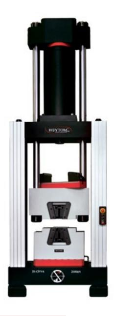
The DI-CP/V4 model, which is part of the PRO series, has been designed to perform tensile, compression, bend/flex and shear testing, with nominal capacities between 400 and 2000 kN. Tension is always tested using the hydraulic grips, located in lower area, and compression in the upper test area.
