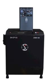
The DI-CP/V2 model, which is part of the PRO series, has been designed to perform tensile, compression, bend/flex and shear testing, with nominal capacity between 1500 and 2000 kN. Tension is always tested using the hydraulic grips, located in lower area, and compression in the upper test area.
