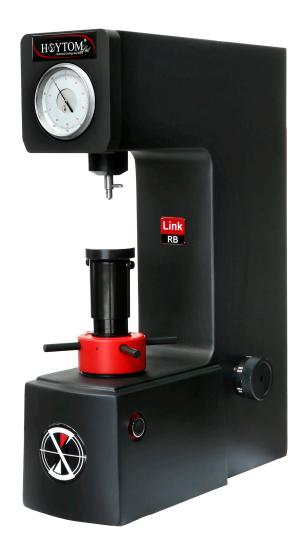
The Link RB model is a Rockwell hardness tester that is capable of applying loads of 60, 100 and 150 Kg. It also has additional loads for Brinell tests (31.25, 62.5 y 187.5 Kg).
