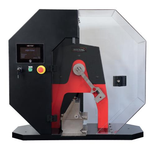
The Hoytom tabletop pendulum impact tester has been designed to test plastics and composites according to the Charpy or Izod impact testing standards.
